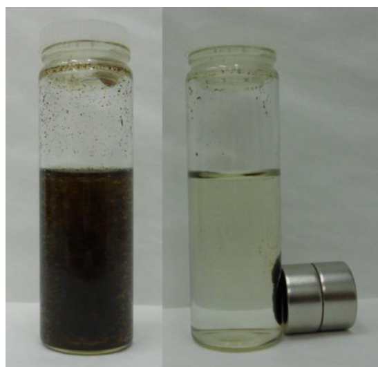
Fig. 2. Demonstration of magnetic separation of magnetic chitosan microparticles prepared by microwave assisted synthesis (MWCH).
